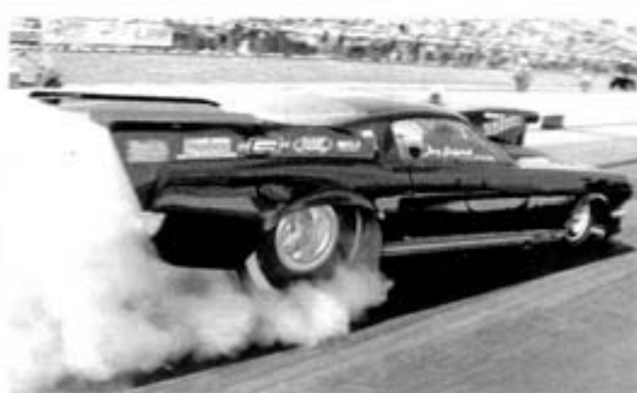
JERRY AND Linda Bridgetorth wanted to build a unique car that nobody had ever built before, so they chose a '66 Shelby GT-350H. While you may say many people have built Shelby look-alikes, however, this has to be the first one to run 6.60s at over 200 mph. The Tim McAmis-built chassis gets right down to business with a Charlie Peppers 705-cube Ford hemi with a mild dose of Gene Fulton-tuned nitrous oxide.
